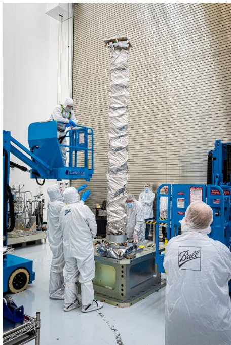
Figure 8: IXPE Flight Boom, First Deployment at Ball
